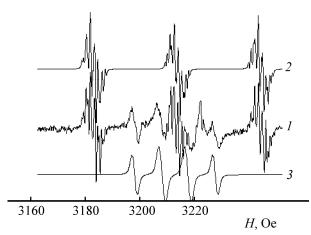
Fig. 4. (1) Experimental ESR spectrum of a mixture of radicals generated by electrochemical oxidation of Dimephosphone oxime (IIg) in acetonitrile in the presence of pyridine (acetonitrile–pyridine ratio 5.0:0.1), (2) theoretical ESR spectrum of iminoxyl radical IIIa, and (3) experimental ESR spectrum of nitroxyl radical generated from IIIa.
